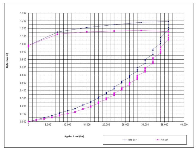
8. The load deflection curve below, obtained from a tension load test, is for a 2-7 /8" O.D. shaft, with 8", 1 O" and 12" helix configuration. The final installation torque was 3,300 ft-lb.
